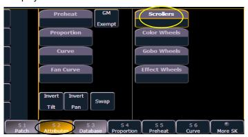
The picker displays on the left half of the CIA when you select the specific attribute ({Scroller}, {Color Wheel}, {Gobo Wheel}, or {Effect Wheel}). The picker displayed is specific to the selected attribute (the scroll picker will display when {Scroller} is clicked, the color wheel picker will display when {Color Wheel} is clicked, and so on).
