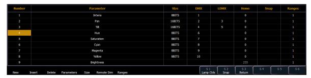
Step 3: Determine the total number of parameters that your fixture has. Do not count 16-bit channels as two channels, this will be done in a later step.
