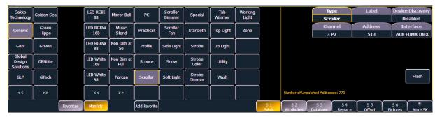
Press **(Manfctr)** from the CIA to display the fixture library. The two columns on the left are pagable and show manufacturer names. Use the arrow buttons to scroll the list of manufacturers. Selecting a manufacturer repaints the device columns with all devices from that manufacturer that are available for patching.
