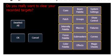
From the **{Clear Targets}** screen you can select which record targets you wish to clear. The buttons at the center of the CIA represent all of the record targets that you can choose to clear. By default all components are selected (gray) and will be cleared. To withhold any targets from being cleared, simply deselect them in the CIA by clicking the respective button.
